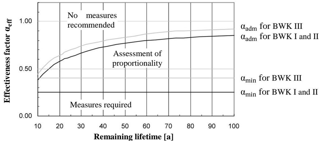
**Figure 2:**  $\alpha_{\min}$  and  $\alpha_{\text{adm}}$  thresholds (cf. SIA 2018 (2004). Fig. 6)
