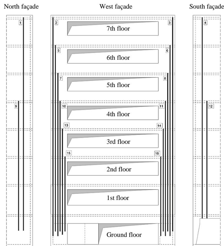
**Figure 6:** Configuration diagram of the post-tensioned strengthening systems
