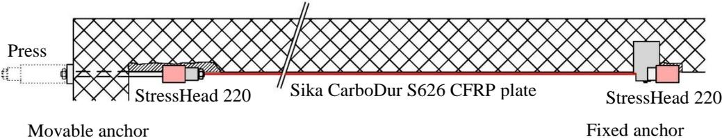
**Figure 4:** Schematic drawing of the StressHead CarboStress post-tensioning system
