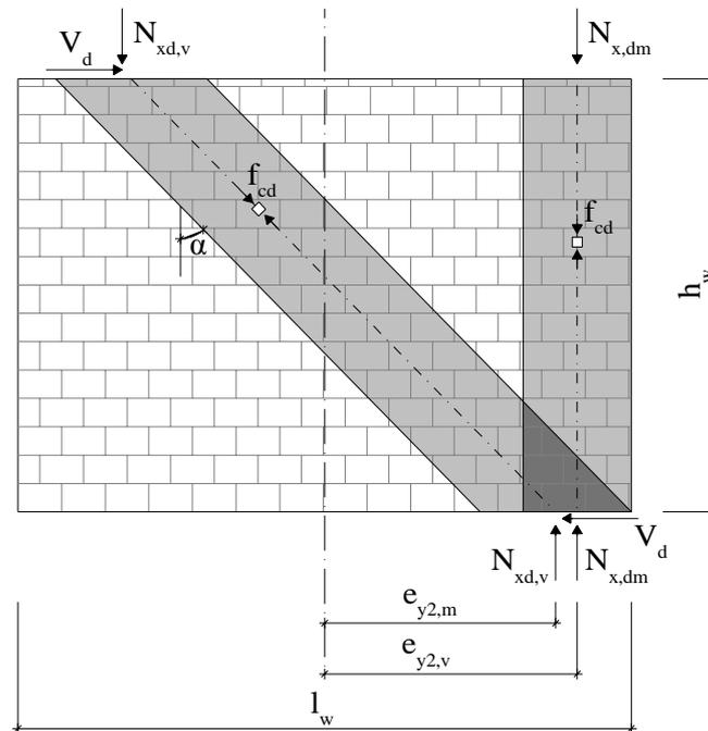
**Figure 3:** Stress fields of the walling system
