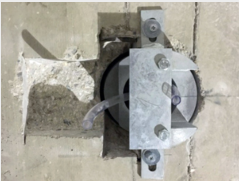
Step 2: Fitting the fixed and movable anchors
